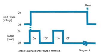
Upon application of input voltage, the relay contacts transfer and a preset delay begins. At the end of the preset delay, the relay contacts drop out and remain in that condition for a second, independently adjustable preset time. At the end of this time, the relay contacts pull in and the sequence repeats until input voltage is removed.
